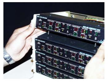
"Stacking" the Lincs distributes power up from the base to the Lincs via the power jacks on each module from the receptacles below. Align the tips of the jacks with the center of the receptacles' openings on the Linc below.
