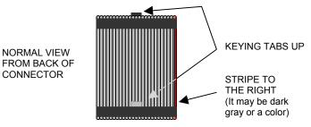
The connectors must be fully seated and the locking tabs on the side must snap securely around the connector shoulder. See the picture on page 7.
