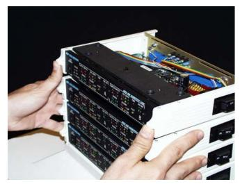
To remove Lincs, **push up on the thumb tab** as shown to apply upward force properly (from the front of the Linc). **Lifting from the back of the Linc will bend the jacks.**
