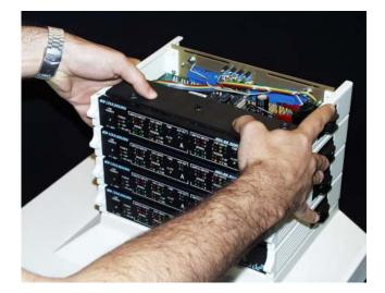
When aligned, push the Linc module down to seat it firmly. After you have installed the Lincs, install the lid on top of the stack to complete the power-safety circuit.
