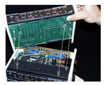
The 4 jacks on the bottom of the Linc plug into the 4 corresponding receptacles on the top of the Linc below. The first Linc mounts on the receptacles on top of the power base.
